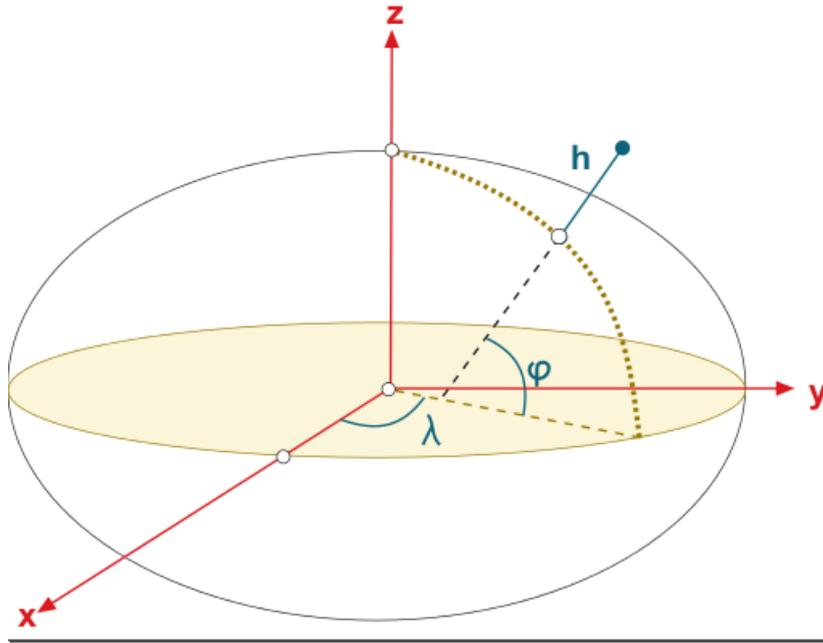
Figure 1: The Cartesian coordinate system in terms of latitude, longitude and height normal to the surface
