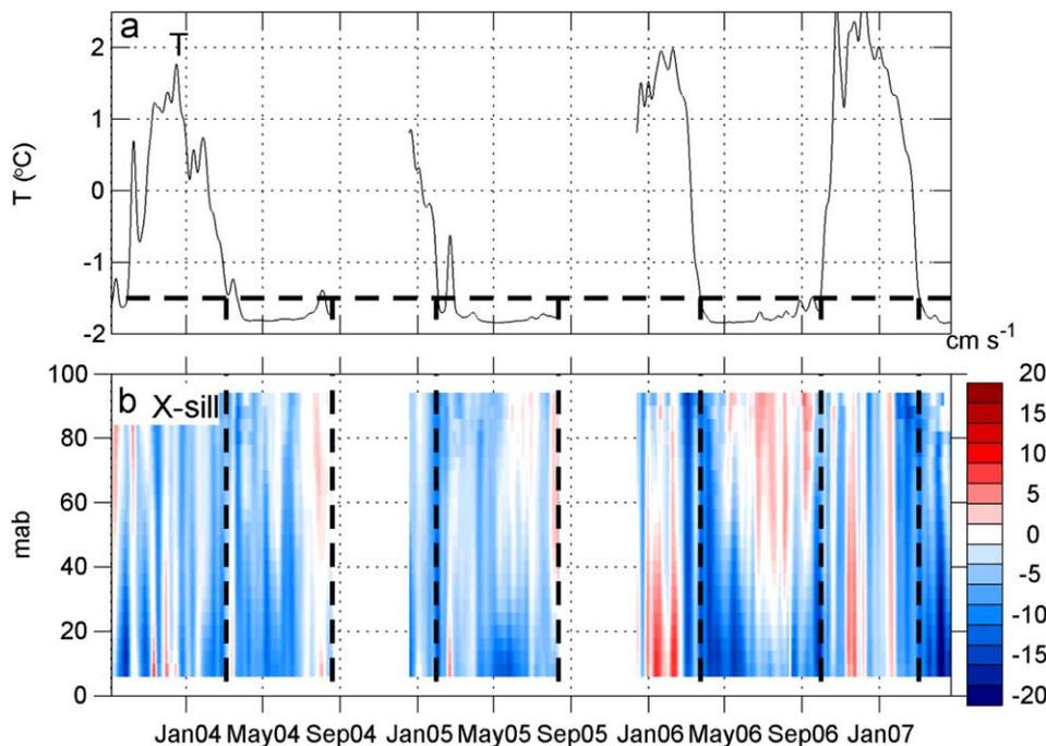
Fig. 3. Time series of (a) bottom temperature and (b) cross-sill component of the velocity (negative values out of the fjord) for the period covering all four deployments. 15-day low-passed hourly data are shown. Vertical dashed lines mark the times of overflow onset and end. Horizontal dashed line in (a) is the upper limit for BSW temperature equal to -1.5 °C.
