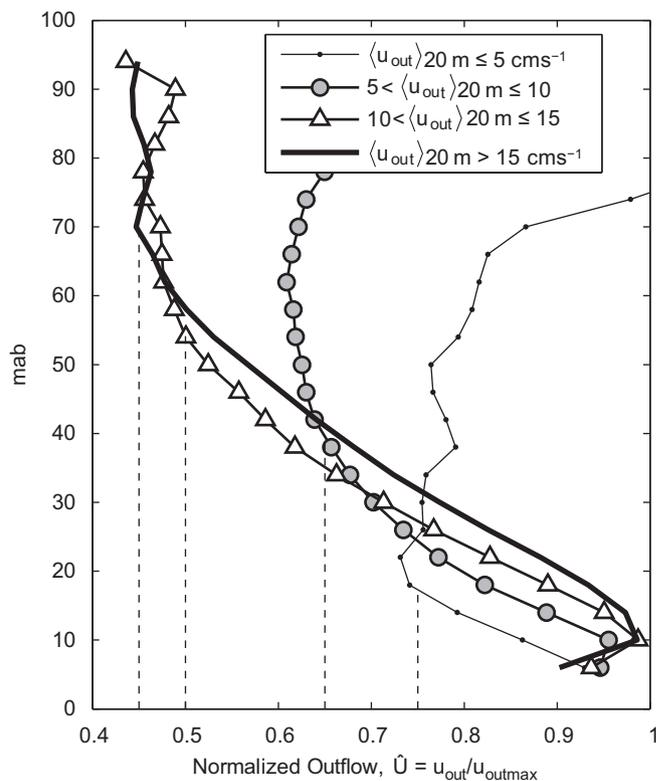
Fig. 2. Profiles of outflow velocity normalized by the maximum outflow in the bottom 20 mab. Ensembles are averaged in  $5\text{ cm s}^{-1}$  bins of the average outflow in the bottom 20 mab. Vertical dashed lines mark the thresholds that are used to determine the plume thickness.
