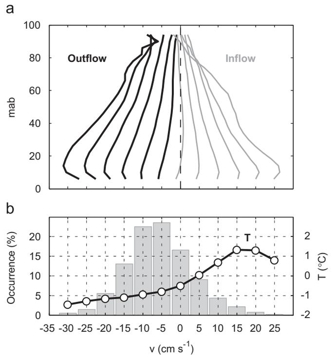
Fig. 4. (a) Average current profiles for the north (cross-sill) component of the velocity grouped according to the 20 mab averaged bottom current in 5 cm s<sup>-1</sup> increments. Black (gray) traces mark outflow (inflow). (b) Histogram of northward bottom current (vertical bars) and the corresponding average bottom temperature for each velocity bin (circles).
